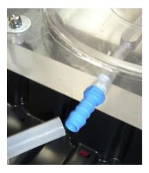
5. Attach the brown plastic pipe, which is already attached to the pump, to the brass valve at the bottom of the Bubble Tube Column.
