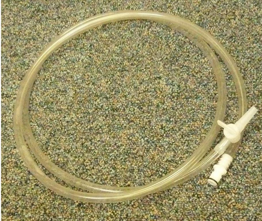
Connect this tube to the white socket on the bubble tube base, next to the POWER IN socket. Push the end with the black stripe into the white socket till you hear a click to indicate that it is secure. Make sure the other end with the tap is in a suitable container to take the water. Turn the tap to release the water.
