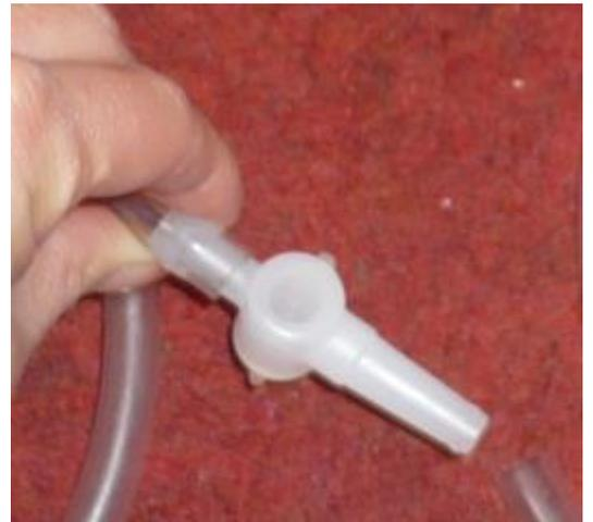
Connecting the filling pump to the bubble tube power supply:
