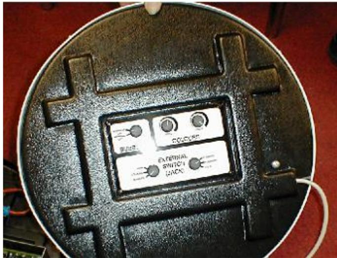
7. With the left hand dial set to BOTH and the right hand one to FLASH ON, then the Bubbles and Lights will be off and they will only come on when the ROMPA<sup>®</sup> switch is activated.
