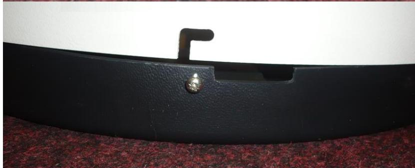
3. The bubble tube column needs to be fitted to the base unit using the four screws provided (shown below on top of silver-coloured washers). Note the location of the valves before screwing in place – orientate the column so the pipes are near to their corresponding valve. See point 5.
