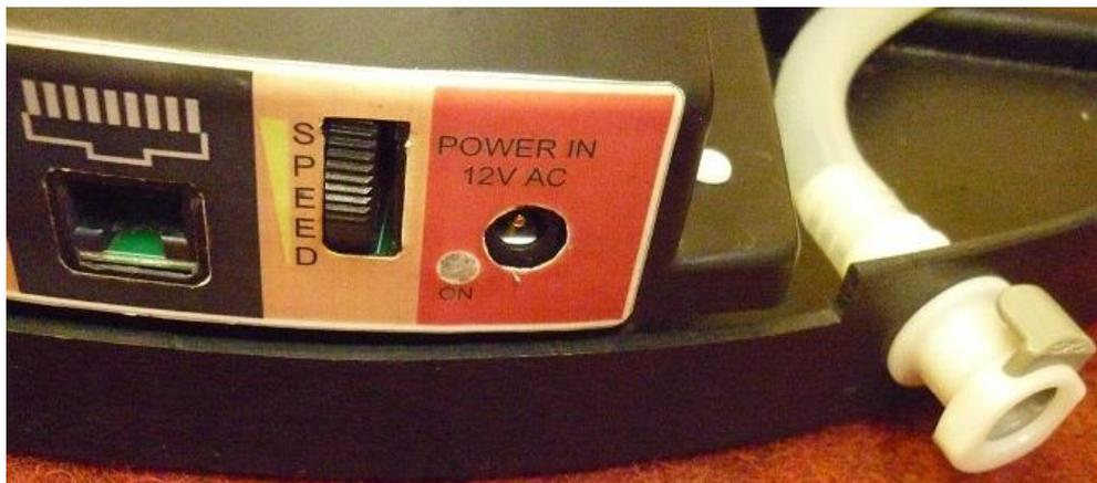
To remove the drainage tube, push on the grey button to release the tube. Removing the drainage tube automatically seals the cloudy pipe of the bubble tube. Empty any water that has remained in the drainage tube. Keep a piece of paper towel to hand to place under the white socket to catch the small amount of water that can be released.
