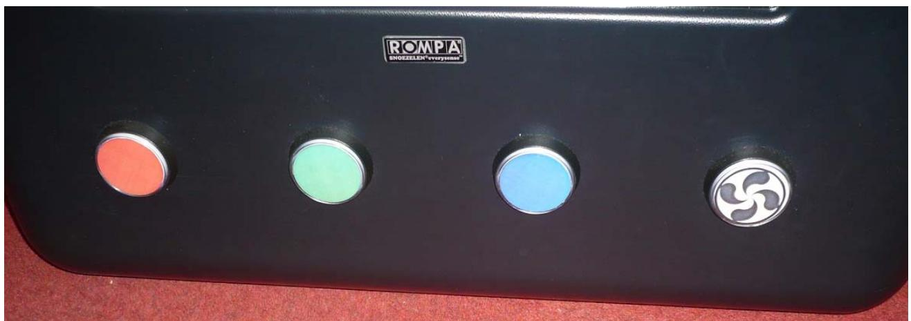
5. The furthest right button controls the fan. This has three settings. With each subsequent press, the speed of the fan increases.
