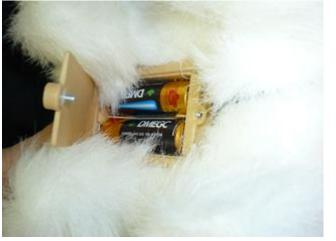
Close the battery compartment and tighten the screw to secure in place.
