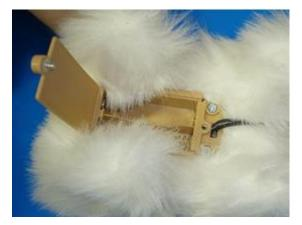
Insert two AA batteries, observing the polarity indicated.
