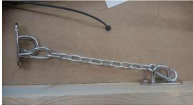
5. Attach a chain to each eye plate, making sure that all the chains are the same length.
