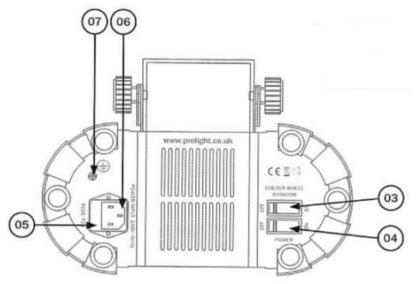
03 = Colour wheel rotation switch 05 = Fuse: F2 250V 04 = On/off switch
