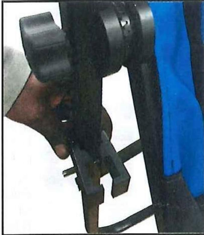
7. Slide the left side of the metal Foot Rest extension assembly into the straight clamp 1" square tube. Then feed the carriage bolt through the right inner hole of the straight clamp 1" square tube and feed through to the outer hole.
