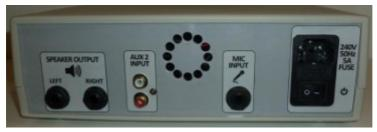
5. Connect the black lead that has a pair of RCA (phono) connectors on each end between the Oscillator and the Amplifier. Connect one end of this lead to the Oscillator. This end is colour co-ordinated i.e. black to black and red to red. The other end of the RCA lead connects to the Amplifier. Connect the two leads with the two mono jack plugs from the speaker box under the Floor to the 6.3mm SPEAKER OUTPUT sockets (LEFT and RIGHT) at the back of the Amplifier.
