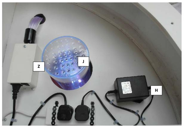
• Check the LED light on the bubble tube chassis. If this is not illuminated, check that the cable to the power socket has not become dislodged during transit. Re-connect as necessary (push in).
