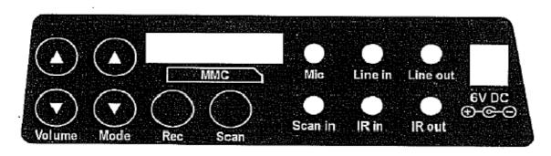
The back of the Paletto features buttons for settings and input and output ports. This is also where the memory card with sounds is to be inserted. The illustration above shows the overlay on the back panel of the Paletto.
