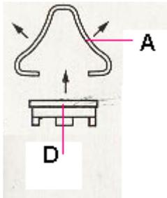
Install a D 1.5V battery or the rechargeable battery 17631 (to be purchased separately). To do this, remove the integral metal loop **A** by pushing the sides of the loop outwards gently. Remove the lid **D**. Install the battery **E**, positive end facing towards the mirror ball and the floor. Replace the lid and metal loop.
