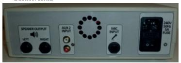
Connect the kettle lead to the socket at the back of the amplifier (top right socket labelled 240V). Switch on using the rocker switch at the back of the amplifier (bottom right). The power indicator light on the front of the amplifier should light up (bottom right hand corner of the front of the amplifier).
