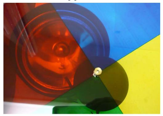
6. Fix the colour wheel with the motor to the pin spot and tighten the screw.
