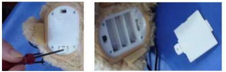
2. Insert three AA batteries, observing the polarity indicated.
