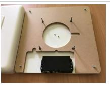
• Gently lift up the tube and place over the base, lining up the 4 screws on the base with the four drilled holes on the square base:
