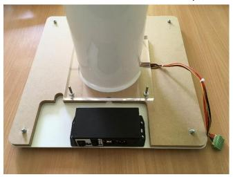
• Secure the tube to the base using the washers and wing nuts provided. Put a washer on each screw first, followed by a wing nut. Twist the wing nuts to tighten:
