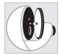
To attach glass-bossed effect wheels (e.g. liquid wheels), tighten the cross-head screw on the shaft of the wheel rotator as shown.
