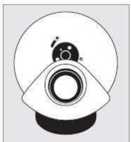
4. To use standard ROMPA® effect wheels with this projector, first remove the magnetic adapter from this projector. To do this, use the small allen key provided and place this in the hole on the top of the magnetic adapter. Twist the allen key anti-clockwise and the adapter will loosen and detach from the projector.
