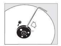
**Please note**: You may have to turn on the projector to move the rotator. The hole on the top of the magnetic adapter must face the top of the projector.
