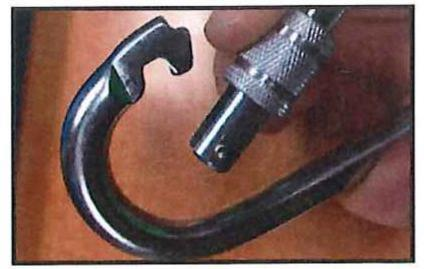
2. The locking nut of the Safety Snap should not move from side to side at any great angle. If it does, discontinue use immediately.
