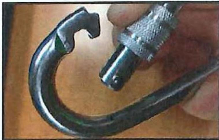
To close and lock the Safety Snap, turn the locking nut anti-clockwise as far as possible. Each Safety Snap is intended for use with one piece of equipment and / or one accessory.
