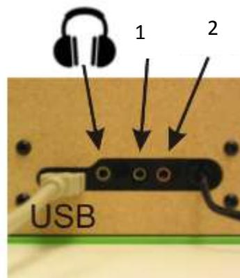
For those with dexterity problems the 'ON/OFF' control and 'NEXT TUNE' buttons can be over-riden by means of remote switches plugged into the two available sockets. The Simple Music Player will accommodate a switch with a 3.5mm adapter.
