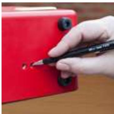
Don't press too hard; you should feel a gentle click like on a keyboard or doorbell. Only after holding the control for 5 seconds the volume will begin to increase or decrease, so it can be set to the appropriate level.
