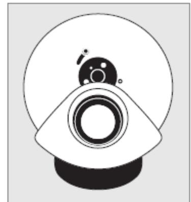
4. To use standard ROMPA® effect wheels with this projector, first remove the magnetic adapter from this projector. To do this, use the small allen key provided and place this in the hole on the top of the magnetic adapter. Twist the allen key anti-clockwise and the adapter will loosen and detach from the projector.
