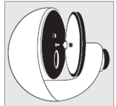
Once the magnetic adapter has been removed, push the wheel onto the shaft of the wheel rotator as shown. A slight twist when attaching the plastic-bossed push on effect wheel will help.
