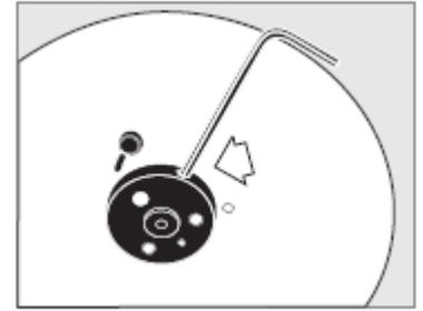
**Please note:** You may have to turn on the projector to move the rotator. The hole on the top of the magnetic adapter must face the top of the projector.
