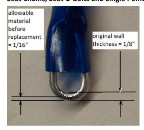
There are three other components that might experience some wear over time; Seat Chains, Seat U-bolts and Single Point Attachment. Wear in these areas are normally very light, but still should be checked. The following images show where to look for the wear and how to gauge the need for replacement. If any are found to have worn half way through the wall thickness, they need to be replaced.
