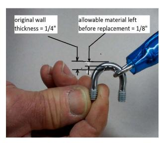
Note: For clarity, the seat u-bolt is shown without the seat. Also, although just one end of the chain is shown above, both ends would have to be inspected.
