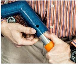
Take one upper leg section and align the short, exposed end with one casting backbone leg section as shown. As mentioned above, the shorter exposed end of the upper leg section is what mates with the backbone leg. Locate the line on the exposed tubing that will assist in alignment.
