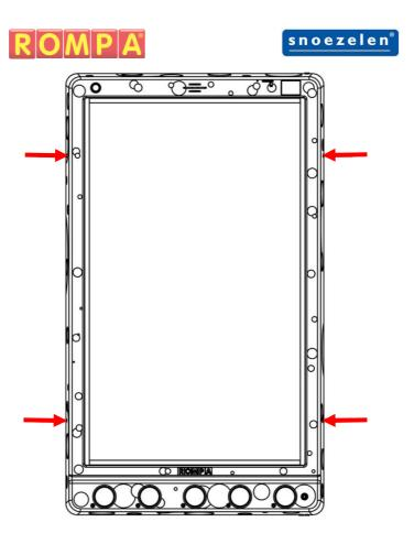
4. Secure both brackets to the wall\* ensuring the centre of the bracket mounting holes line up with the marks just made to ensure the bracket it level when mounting it to the wall. The top bracket mounting holes should line up with the top 2x marks and the bottom bracket mounting holes should line up with the bottom 2x marks.
