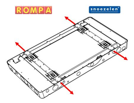
Unscrew the 4x M4 screws which secure the 2x brackets to the panels. The brackets are secured to avoid any damage during transit.
