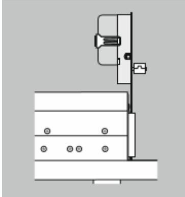
Plug the round tip of the 12V transformer into the 12V socket on the rear panel. Plug the 12V transformer into a mains socket and switch on at the wall.
