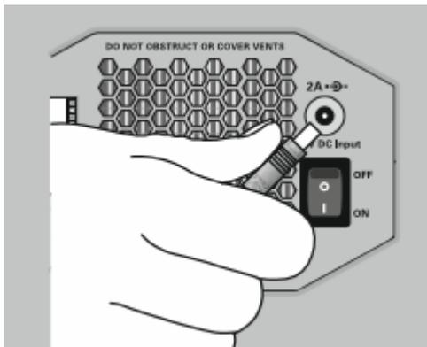
Then turn the projector on by the mains switch to the "I" (ON) position. "O" is the OFF position.
