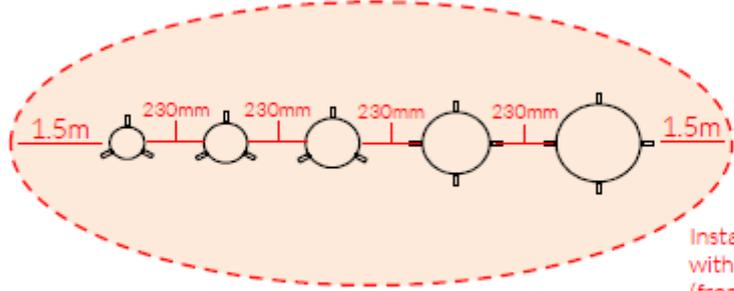
Install Instrument with 1.5m free space (from widest point) around it.
