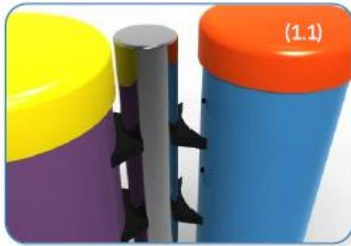
2. Attach Ground Fixings to legs (1.2) (See Ground Fix Post Installation Sheet)
