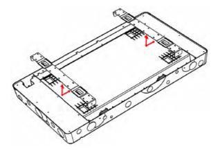
3. Hold the panel where you would like it to be mounted ensuring it is level. Whilst in position mark where the centre of the bracket mounting holes are on the wall. Do this for all 4x bracket mounting holes.
