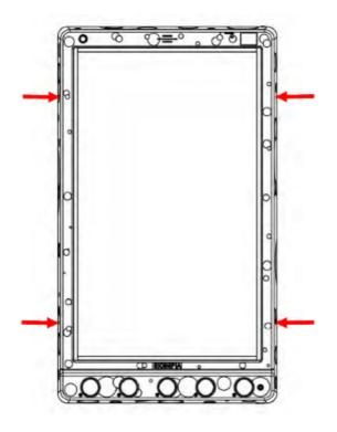
4. Secure both brackets to the wall\* ensuring the centre of the bracket mounting holes line up with the marks just made to ensure the bracket is level when mounting it to the wall. The top bracket mounting holes should line up with the top 2x marks and the bottom bracket mounting holes should line up with the bottom 2x marks.
