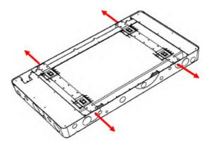
1. Unscrew the 4x M4 screws which secure the 2x brackets to the panels. The brackets are secured to avoid any damage during transit.
