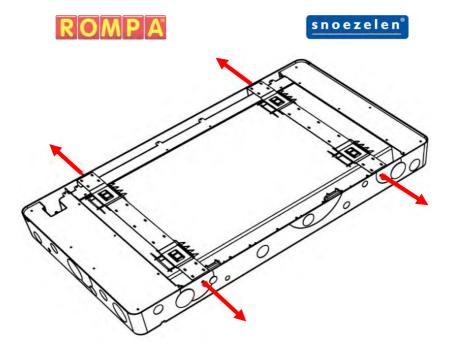
1. Unscrew the 4x M4 screws which secure the 2x brackets to the panels. The brackets are secured to avoid any damage during transit.
