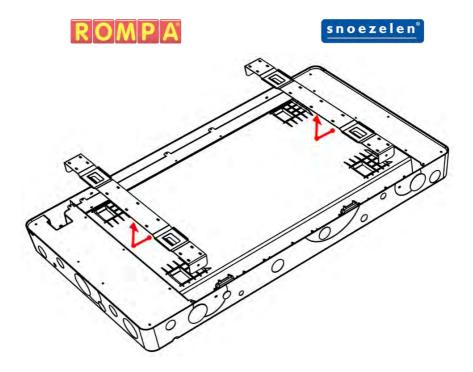
3. Hold the panel where you would like it to be mounted ensuring it is level. Whilst in position mark where the centre of the bracket mounting holes are on the wall. Do this for all 4x bracket mounting holes.
