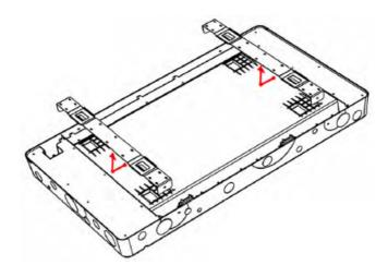
3. Secure both brackets to the wall\* ensuring the centre of the bracket mounting holes line up with the marks just made to ensure the bracket is level when mounting it to the wall. The top bracket mounting holes should line up with the top 2x marks and the bottom bracket mounting holes should line up with the bottom 2x marks.
