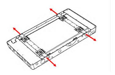
Unscrew the 4x M4 screws which secure the 2x brackets to the panels. The brackets are secured to avoid any damage during transit.
