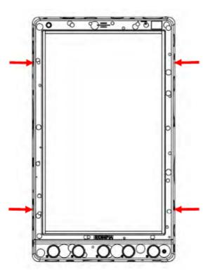
4. Secure both brackets to the wall\* ensuring the centre of the bracket mounting holes line up with the marks just made to ensure the bracket is level when mounting it to the wall. The top bracket mounting holes should line up with the top 2x marks and the bottom bracket mounting holes should line up with the bottom 2x marks.
