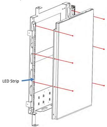
Please ensure all tubes, wires and LED strip (position from its sides) do not get trapped or damaged.
