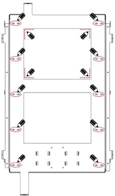
4. Drill a minimum of 6 x M6 holes in your marked screw positions
