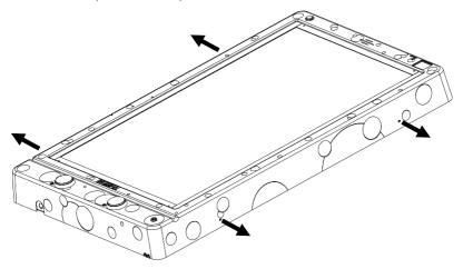
Next remove the framework from the TOP of the panel where the touchscreen locates, as shown the illustration below.
