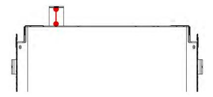
9. Plug the External Power Supply to the cable located at the bottom of the bracket.
